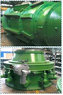
Axial and mix-flow one-stage semi submercible pumps equipped with control system hydro characteristic
